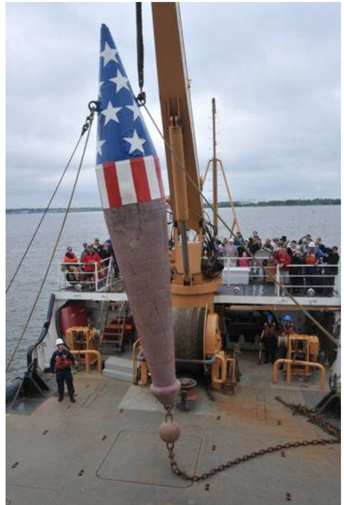
BALTIMORE - The Coast Guard Cutter James Rankin, a 175-foot buoy tender homeported in Baltimore, lifts the Francis Scott Key buoy off the deck in order to lower it to its location in the Patapsco River, May 24, 2010.
